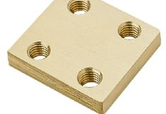
The Short D Plate (Part # 80329001) is made of brass and fastened to the back of a single cylinder MD Series Type D interlock to allow front mounting (see MD Series Data Sheet 1.4). The thickness of the Short D plate is 3/8". To order this plate with your MD Series Type D interlock, put the letter "P" in column fourteen of the interlock part number - reference the MD Series Ordering Guide.
