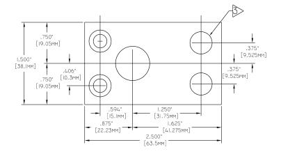
NOTES: 3) .406" (10.32mm) dia. holes for mounting bolts (2 holes). 4) When ordering the FN Plate, consider adding 1/4" to the MD Series Type FN locking bolt length to compensate for the thickness of the FN Plate.
