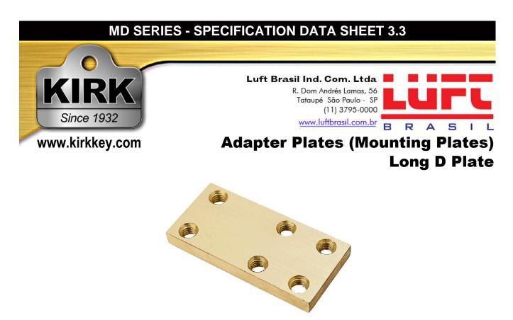
The Long D Plate (Part # 80329002) is made of brass and fastened to the back of a multicylinder MD Series Type D interlock to allow front mounting (see MD Series Data Sheet 1.4). The thickness of the Long D Plate is 3/8". To order this plate with your multi-cylinder MD Series Type D interlock, put the letter "P" in column fourteen of the interlock part number reference the MD Series Ordering Guide.
